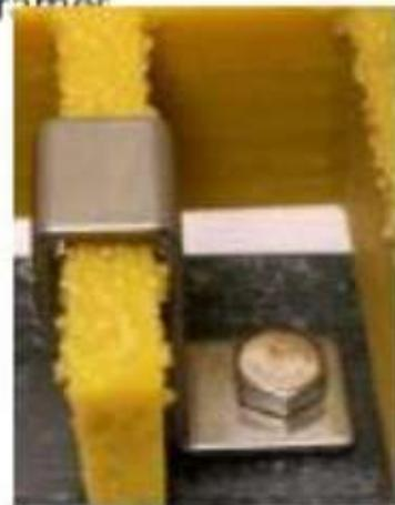
Type **"G"** stainless steel hold clips designed to attach grating to any structural member flange, 3/4" or smaller in thickness, with no drilling required.
